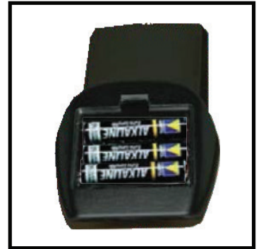
Fig. #64 Remote Control Transmitter battery bay
