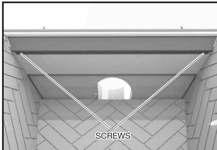
Figure 52: Side panel retainer location.
