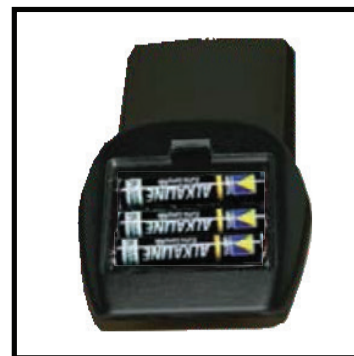
Fig. #61 Remote Control Transmitter battery bay
