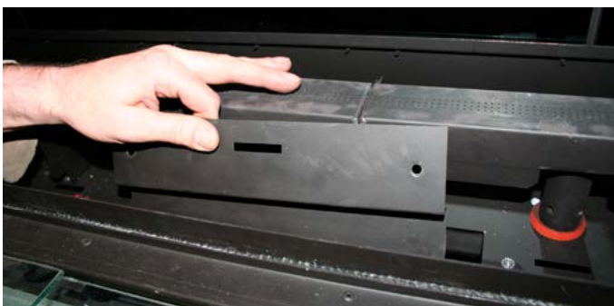
Figure 36c. Remove 4 screws and then remove gas connection cover.
