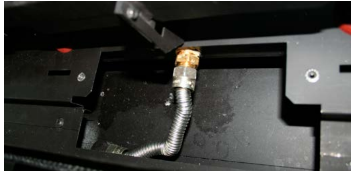
Figure 36d. Disconnect the flexible gas connection line.
