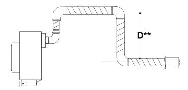
Figure 12b. Multi-Elbow with downward vent run, Top orRear Vent,Wall mounted power vent.
