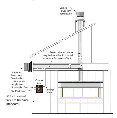
Figure 15. R520\* Series Control Box / Power Vent Wire Routing Diagram
