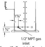
Figure 17. Gas Inlet Supply location.
