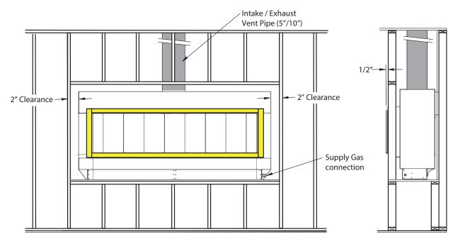
Figure 4. Fireplace installation, (Inlet Gas & Power Vent).
