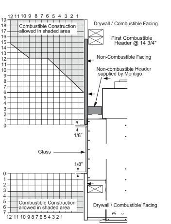
Figure 20. Combustible mantles and facings. (Not to scale)
