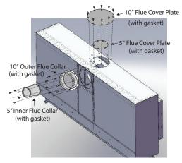
Section 3-1: Converting to Rear Vent
