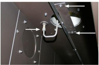
**Figure 9.** Removal of Top Vent air baffle and pressure sensing tube.
