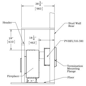
Figure 2c. Clearances for straight rear vented installation with PVHFL510-300.
