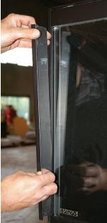
Step 3: Remove the trim from the bottom of the door as shown.
