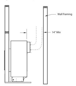
Figure 2. Clearances for rear vented installation with elbow.
