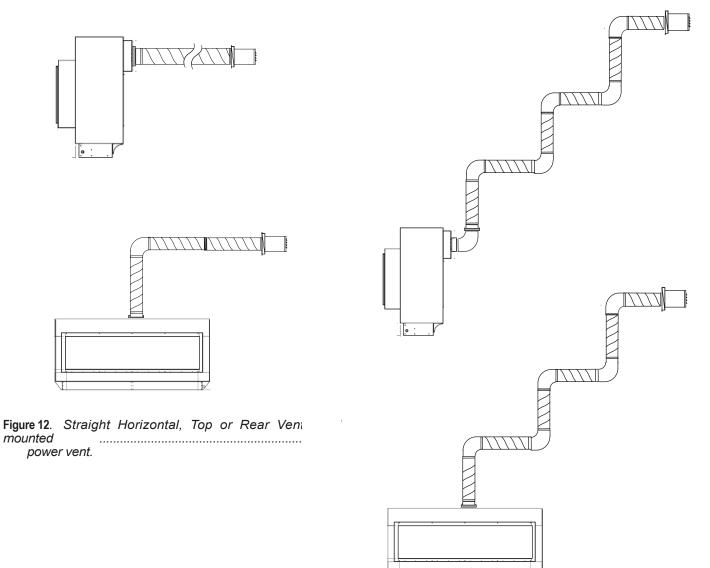
Figure 12a. Multi-Elbow, Top or Rear Vent, Wall mounted power vent.
