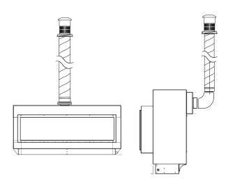
**Figure 10.** Straight Vertical, Top or Rear Vent, Roof mounted
