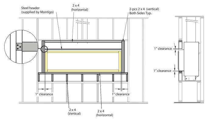
Figure 5. Completed back frame Fireplace installation
