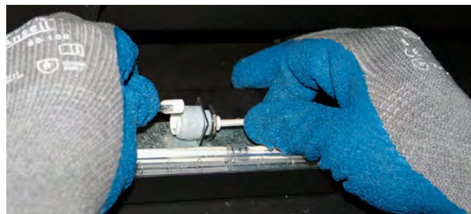
Figure 29a. Wear gloves when handling light bulbs. To remove a light bulb, pull connecting wire away from bulb and pull light bulb up. Replace with new light bulb.
