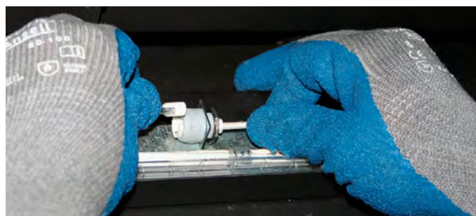
Figure 30a. Wear gloves when handling light bulbs. To remove a light bulb, pull connecting wire away from bulb and pull light bulb up. Replace with new light bulb.
