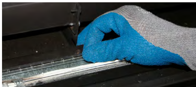
Figure 30b. Rotate newly replaced bulbs in a full circle. Place glass cover back in the burner tray.
