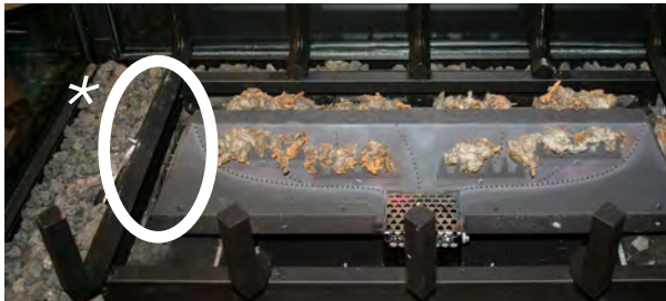
Figure 27. Place the provided embers in the 5 pronged ember holders. Be sure to not directly cover any of the burner holes.
