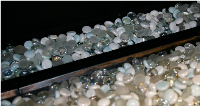
Figure 27. Completed firestone installation. Second Gen burner shown.
