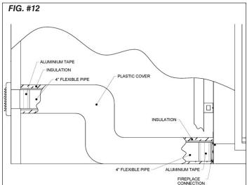
WARNING: THE COMBUSTION AIR INLET MUST BE AT LEAST 5ft BELOW CHIMNEY OUTLET AND MUST NEVER TERMINATE IN ATTIC SPACES OR GARAGES.
