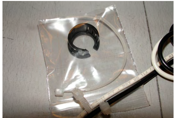
Figure 9 Sec.4 Suppled electrical strain relief and zap strap
