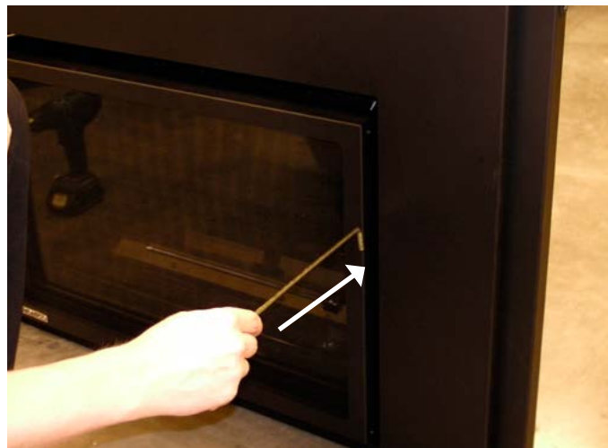
Figure 25 Sec.6 Inserting door tool through the front of the fireplace
