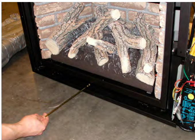
Figure 5 Sec.10 Using the door tool to operate the aeration setting.
