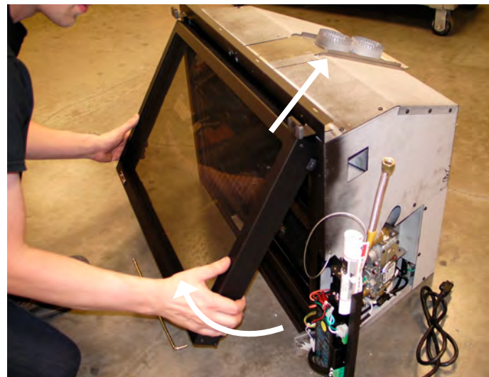
Figure 4 Sec.5 Swing the Door away from the unit, lift over the retaining tabs on top of the firebox. Be careful to not roll the gasket up off the glass when reinstalling the door. Installation is the reverse of removal.
