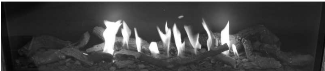
Figure 7: Burner flame appearance Centre Fire
