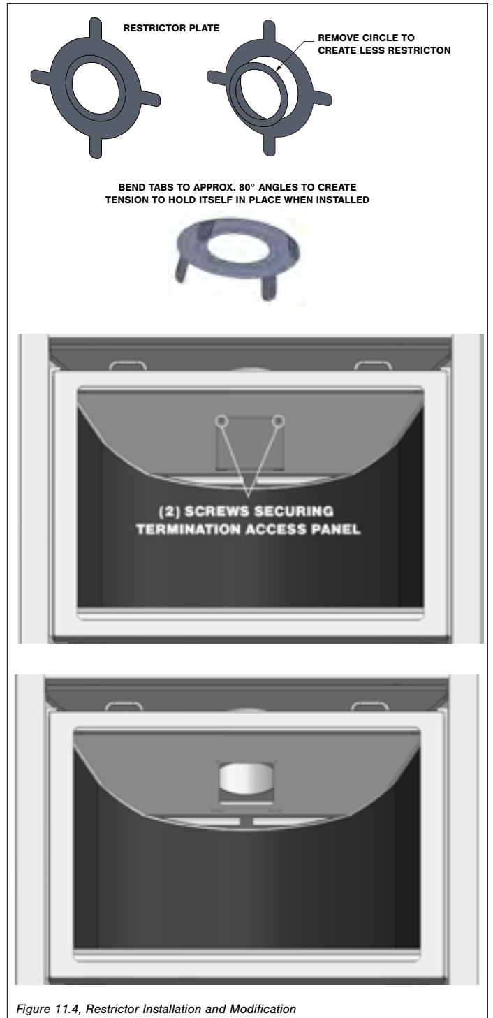
Figure 11.4, Restrictor Installation and Modification
